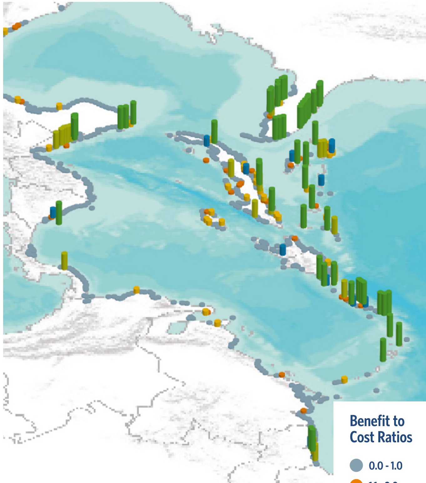
Figure 10 Benefit to Cost Ratios for Private Property Benefits of Mangrove Restoration. This map considers only the flood reduction benefits in averted damages to private property across the Caribbean. Values are the net present value of restored mangroves as an infrastructure asset assuming a 30-year project with a 4% discount rate.
